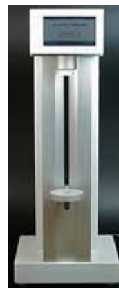
Pic. 26. Lifting arm in start position for the “Manual” mixing program
